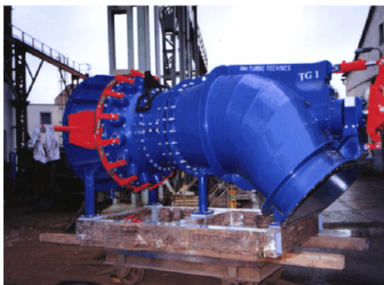
Figure 2 – Example of a Kaplan S Turbine
