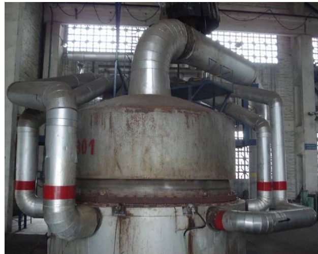
Figure 2. The ammonia burner with the installed de-N 2 O catalyst Figure 3. The existing ammonia burner at the plant
