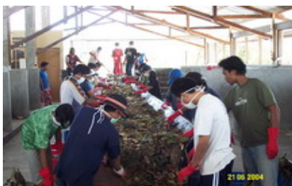
Waste separation conveyer belt
