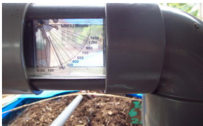
Self-made flow meters
