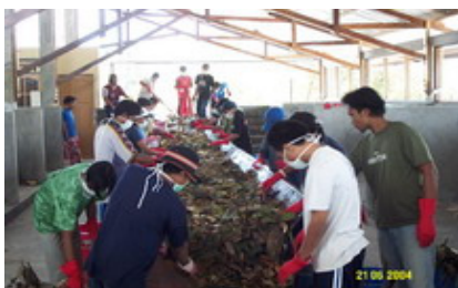
Waste separation conveyer belt
