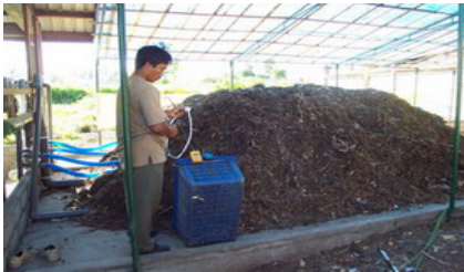
Traditional piles, where the air distributes in 2 dimension yielding very uneven conditions
