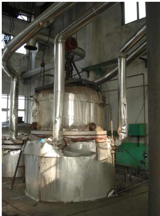
Figure 2. The ammonia burner with the installed de-N 2 O catalyst
