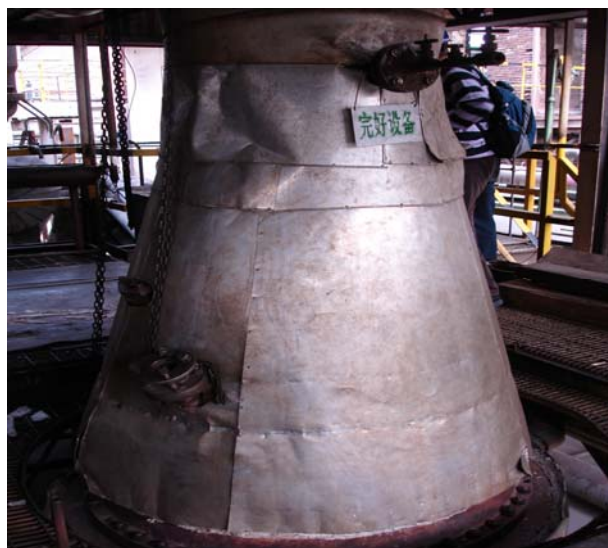
Figure 2. The ammonia burner with the installed de-N 2 O catalyst
